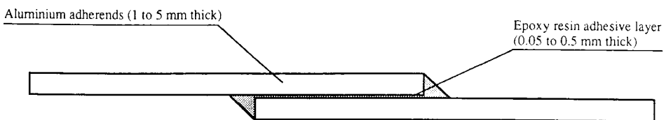
FIGURE 1 Typical aerospace geometry joint.
